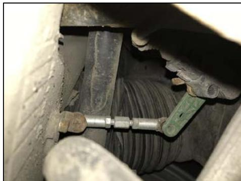
Example of a defective level sensor.
