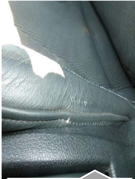
Driver's seat bottom damaged during entry
