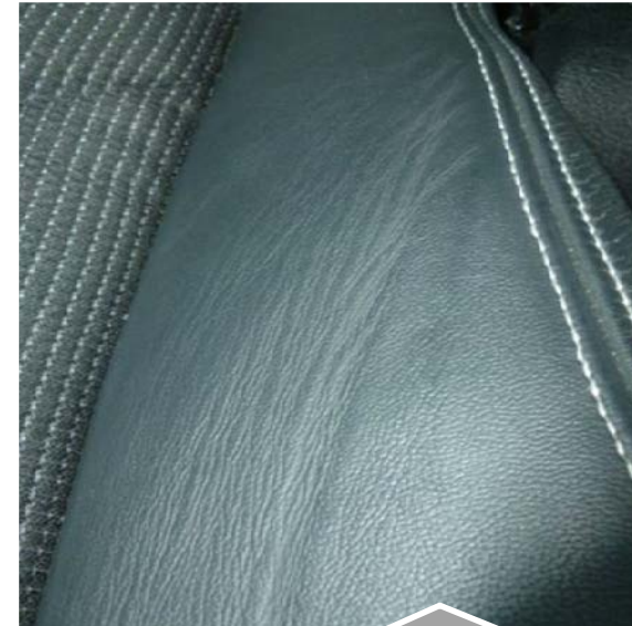
Seat bolster damaged during entry
