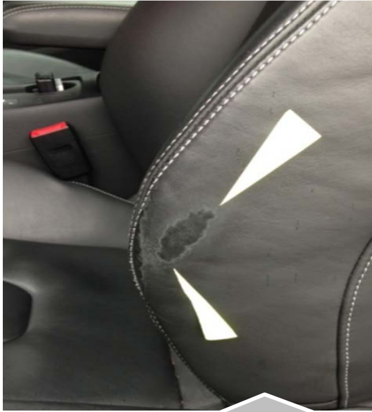
Driver's seat damaged during entry
