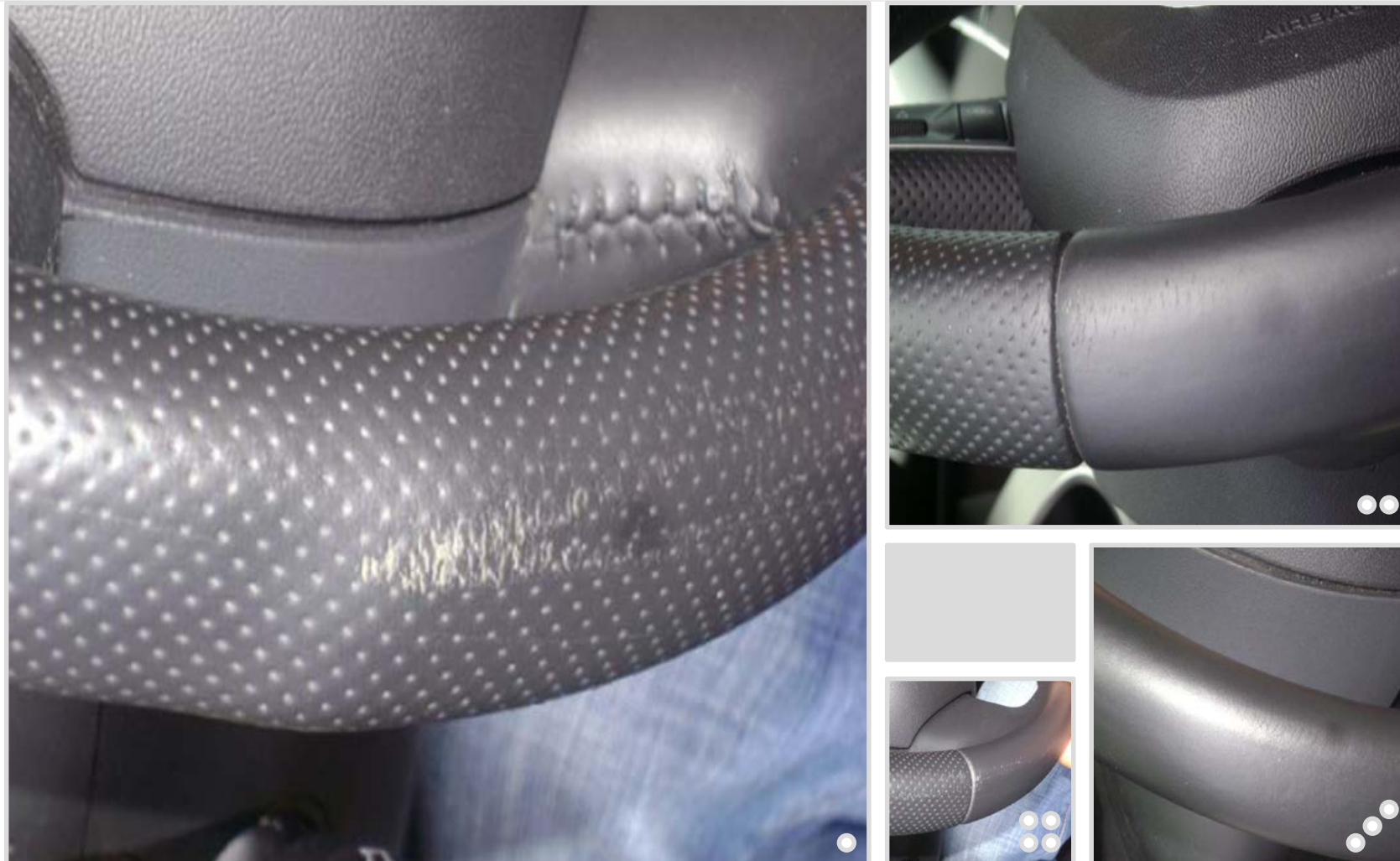
Steering wheel finish abrasion caused by sharp objects, e.g. rings and jewelry
