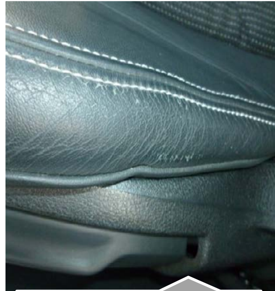
Seat surface damaged during entry
