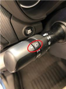
**Step 3)** With the headlights switched all the way ON as shown above (not to Auto), turn the ignition ON and within 10 seconds, cycle the headlight switch from ON to OFF then back ON again 5 times. Observe on the 5th cycle, the headlight beams will raise and dip slightly then re-center.
