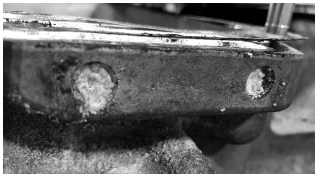
Clogged vent ports
