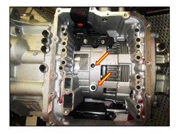
15. Align the manual shaft to the shift lever and install the valve body.
