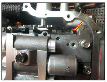
16. Install the valve body bolts and torque the bolts in order from the innermost bolts to the outermost bolts.
