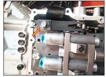
Reconnect the solenoid harness to the solenoids and install the oil temperature sensor.
