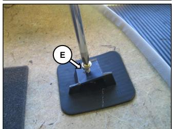
6. Assemble screw (E) into the supplied new clip (F) and fully tighten to base.
