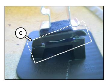
4. Remove broken base clip (C) and remove excess plastic to ensure base (D) is flat.
