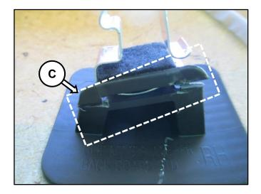
4. Remove broken base clip (C) and remove excess plastic to ensure base (D) is flat.
