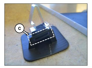
When removing, ensure not to damage bottom seat back retention hooks.
