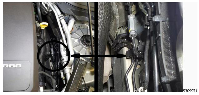
1. Inspect the brake pipe near the steering column as shown. If the brake pipe is secured properly in the clip as shown, no further action is required.
