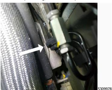
• If the brake clip is missing, install a brake clip.
