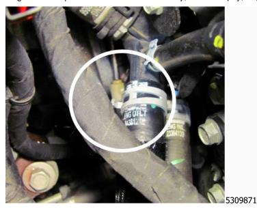
On Malibu (LFV engine) applications only, inspect the engine wire harness adjacent to the heater inlet hose for contact with the heater inlet hose clamp on the engine outlet portion of the hose as shown.
