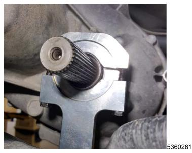
2. Install DT-51329-A on the transfer case front output shaft seal slinger as shown above.
