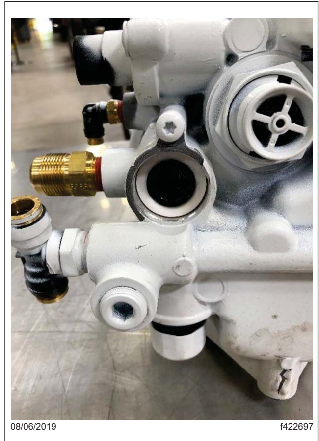
Fig. 3, Plastic Cover Removed
