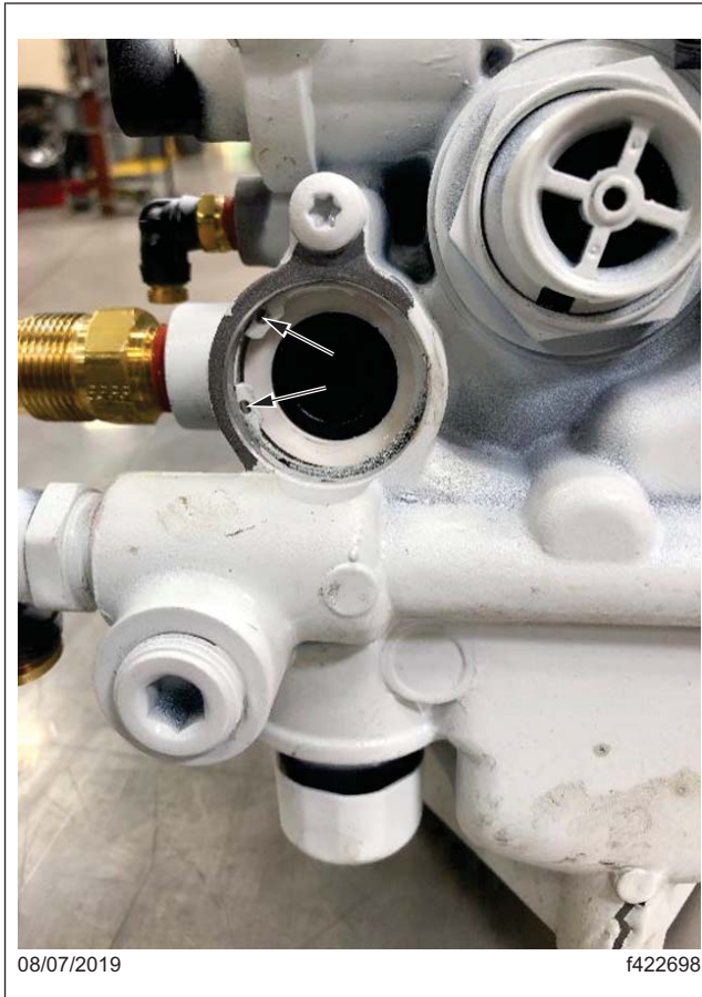
Fig. 4, Snap Ring Installed
