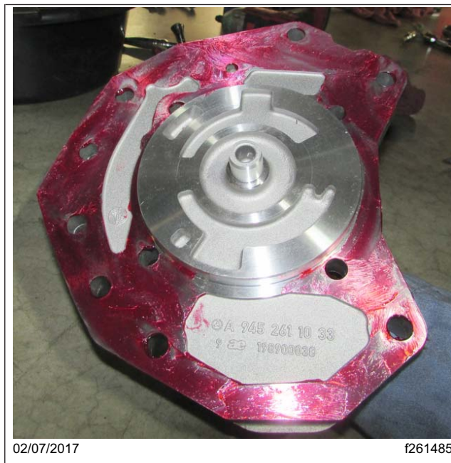
Fig. 12, Sealant Applied to Pump Cover
