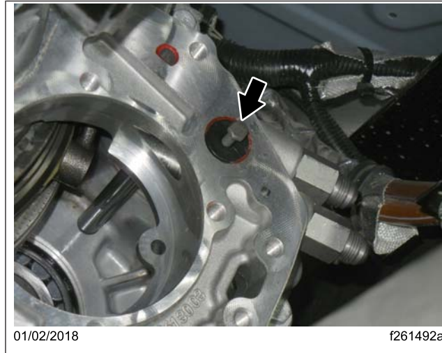
Fig. 10, Original Control Valve
