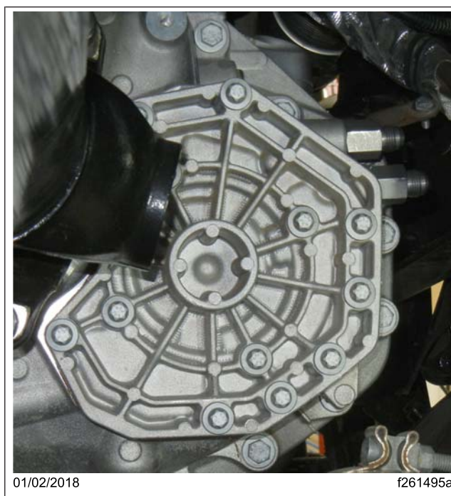
Fig. 9, Transmission Pump Cover
