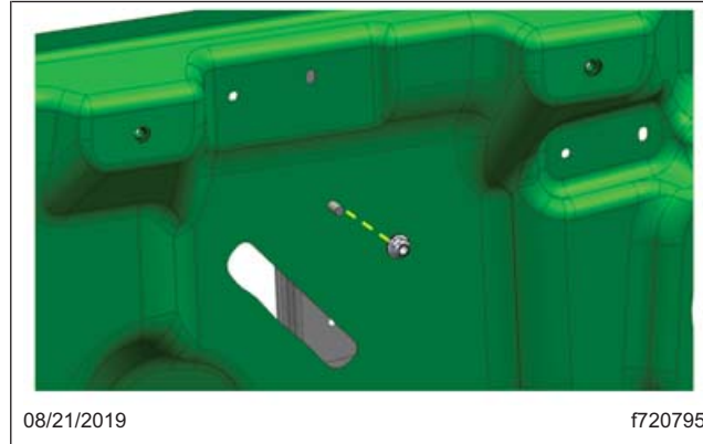
Fig. 11, Nut Fastening Regulator Assembly to Upper Inner Door Panel
