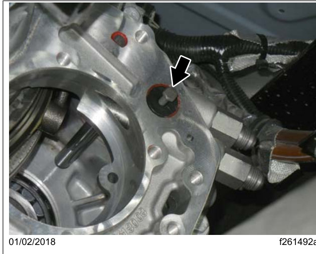
Fig. 10, Original Control Valve
