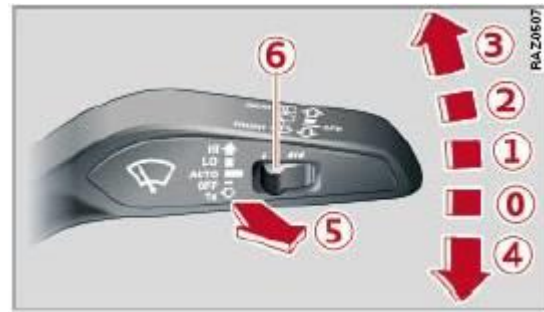
Figure 2. Windshield wiper operating modes.
