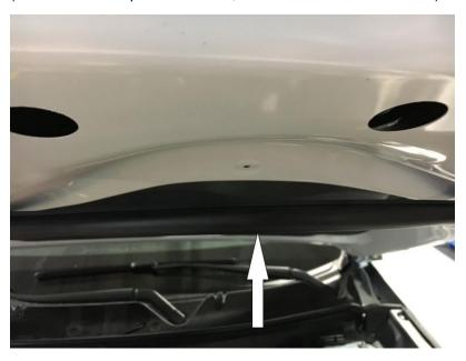
To correct this concern, reattach the weatherstrip or replace it with a new one if it is damaged.
