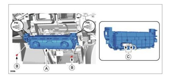
7.(FOR TYPE A VEHICLES ONLY) Replace the rear climate control unit (A) with a modified one according to the instructions on MGSS online (REAR CLIMATE CONTROL UNIT REMOVAL/INSTALLATION). Rear ventillator grille (B).
