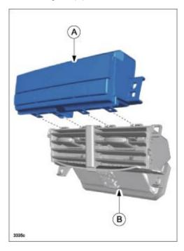
8. (FOR ALL VEHICLES TYPES) Replace the side ventilator grills (A) with modified ones according to the instructions on MGSS online (VENTILATOR GRILLE REMOVAL/INSTALLATION).
