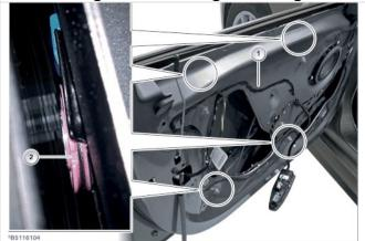
2. Lubricate the rollers (2) of the front window regulator as shown to the left using adhesive grease PN 81 22 9 407 629.
