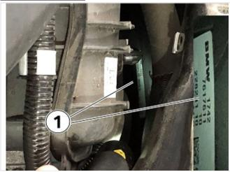
In conjunction with replacing the radiator, check the part number of the fan shroud (1).
