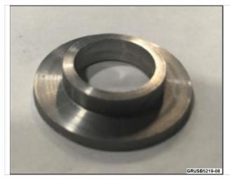
As of CW40 production, one machined washer (shown) will be added to the bottom of the inner seat rail on the passenger's side (right rear) of the 60/40 split 2<sup>nd</sup> row seat.
