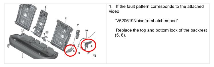
4. Squeaking noises from the rear seat bench (left and right) when loaded.
