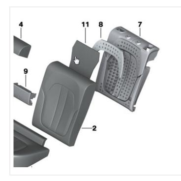
1. Remove the seat cover of the rear seat bench and replace the foam part(s) of the seat if the spring wire at the top of the seat foam is detached and visible (7, 8).
