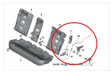
1. Renew the Bowden cable in the luggage compartment and ensure that it is routed correctly (10).
