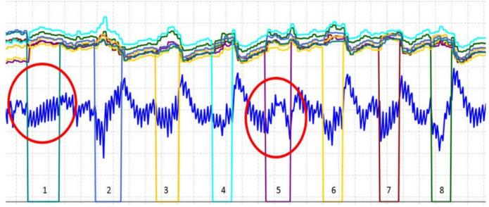
During this final test, it appears that cylinder #5 is not contributing as well as #1. This is one of the main reasons that we must repeat the test to find consistency.
