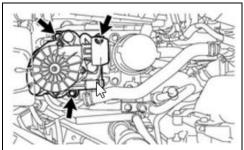
c. Remove the 3 bolts and air pump with bracket.
