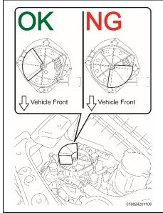
c. Install the **NEW** air pump filter.
