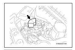
b. Remove and discard the air pump filter.
