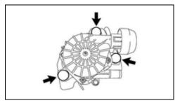
e. Detach the 3 fittings of the air pump insulator and remove the air pump from the bracket.
