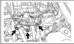
c. Remove the 3 bolts, valve assembly, and gasket.
