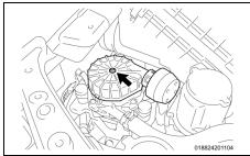
e. Using a Torx T25 socket, install the **NEW** air pump filter cover sub-assembly with the **NEW** hexalobular tapping screw.
