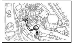
b. Disconnect the air pump connector and detach the wire harness clamp.
