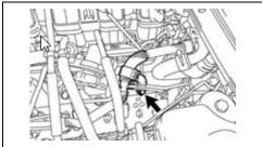
d. Connect the wire harness clamp bracket with the bolt.
