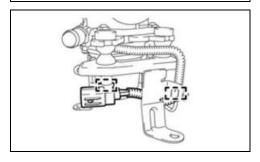
d. Detach the 2 air pump connector clamps.
