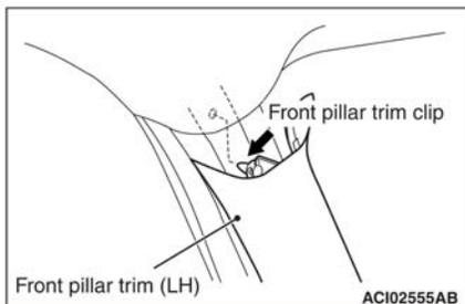
2. Make sure to insert the front pillar trim clip on the upper part of the front pillar trim to the hole on the body.
