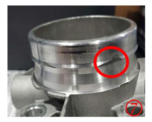
When the charge air cooler outlet tube has become disconnected from the throttle body, the tube end should be inspected for contact damage or a missing O-ring seal from blowing off. If the tube is found to be damaged or the O-ring seal is missing replace the tube assembly. Use the vehicle identification number (VIN),SI, and the GM Electronic Parts Catalog to determine the correct part to order.
