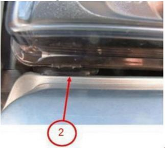
Closer inspection of this area may reveal an improperly positioned front fascia in relation to the head light capsule. Refer to (2) in the image above.
