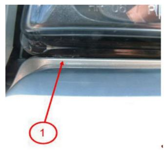
Reposition the front fascia to cover the headlight lower mounting tabs. Correct appearance shown called out as number 1 in the image above. Test drive the vehicle to be sure the vehicle was repaired.
