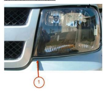
Some customers may comment of a wind noise from the front of the A-pillar, either of the outside rear view mirror(s), or the front of the vehicle. Typically the noise occurs at speeds above 55mph. The source of this noise may be from the headlamp area called out as number
