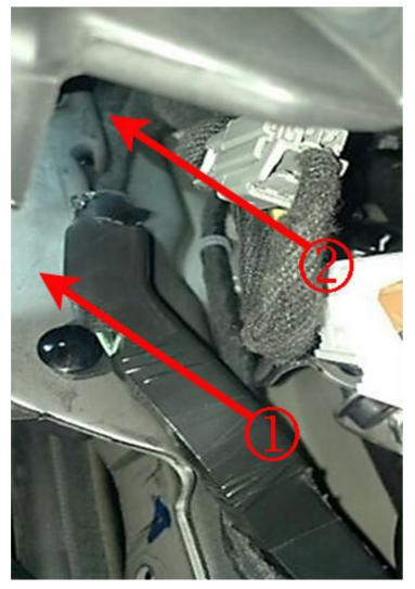
As shown below, the wiring harness (3) is pinched at the lower portion of the left I/P mounting bracket (1). For reference only, call out (4) is the parking brake pedal.
