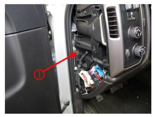
As shown below, the wiring harness (2) is pinched at the upper portion of the I/P mounting bracket (1). In many cases, the complete harness may not be pinched and it can be difficult to see that the harness is damaged. When inspecting for a pinched harness, make sure the harness can be moved freely away from the bracket to body interface.
