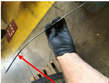
Shaping Stainless Strip to fit contour to windshield opening
