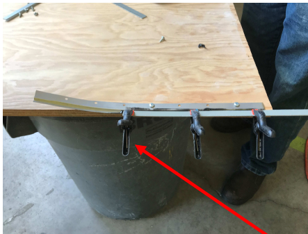
Attaching the fiberglass strip to the stainless-steel strip
