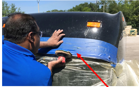
Using a DA sander to remove material to tape line material
