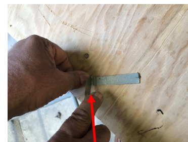
Scoring Fiberglass Strip to fit contour of the windshield opening
