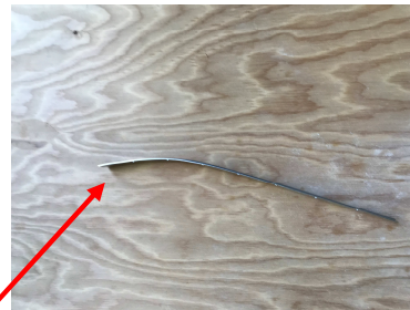
Shaping Stainless Strip to fit contour to windshield opening
