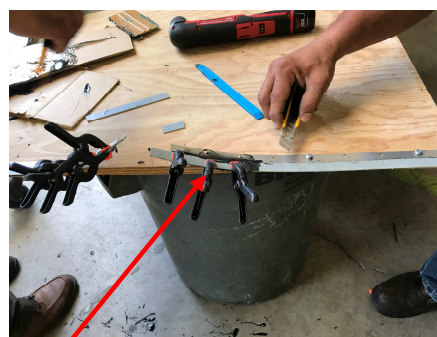
Attaching the fiberglass strip to the stainless-steel strip
