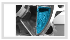
Using a suitable tool install the transmission insert into the area shown and apply an even layer of Devcon putty to the transmission insert until it is completely filled and covered.
