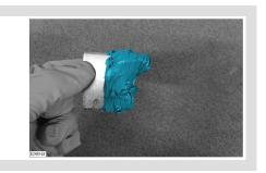
Use a suitable tool apply a layer of Devcon to the transmission insert.
