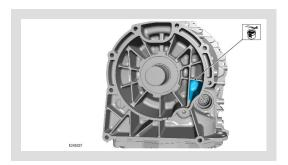
Apply an even layer of Devcon putty to the highlighted area of the transmission.
