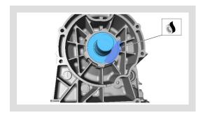
Apply suitable protective tape to the highlighted area of the transmission.
