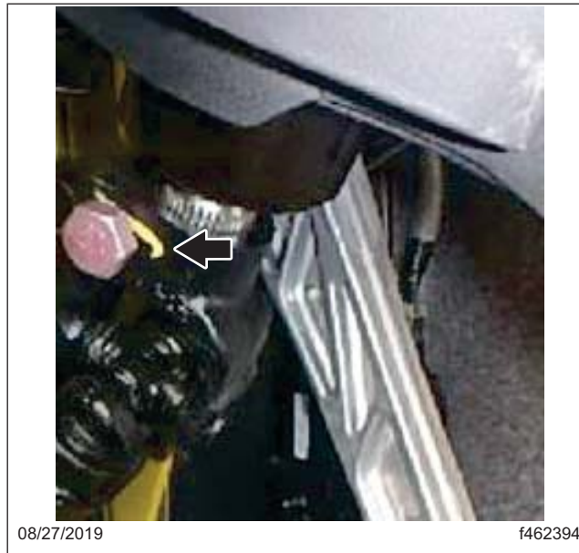
Fig. 1, Bolted Connection Between the Steering Column and the Steering Shaft
