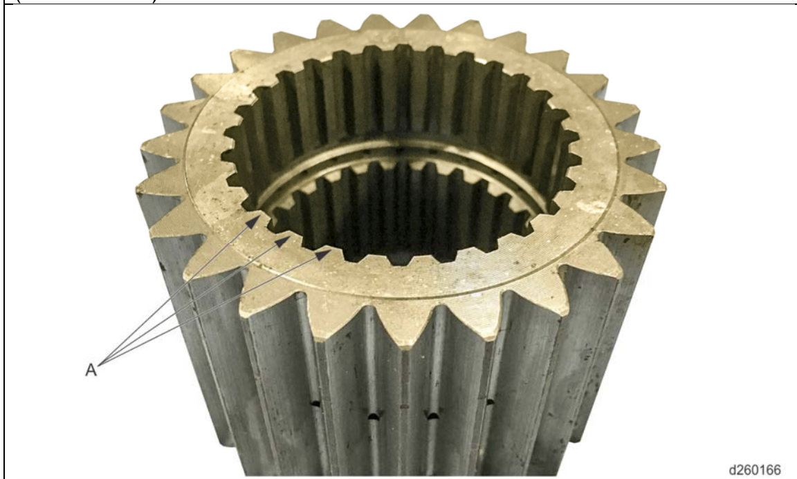
Figure 9 – Sun Gear With The Flat Side Facing Out Towards The Snap Ring Groove
