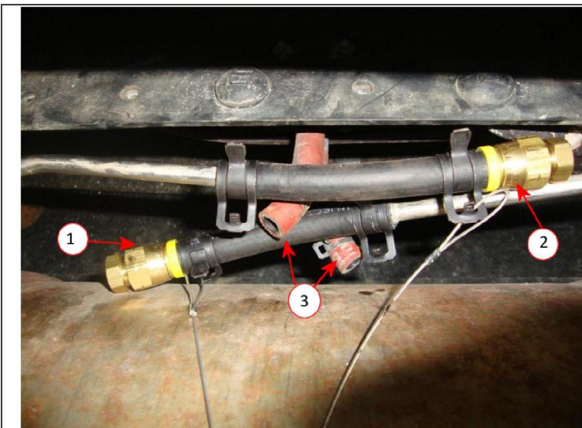
**Photo 3 - EGDP Plugs and Hoses Installed on Steel EGDP Tubes**
