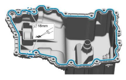
**5.** Install the new oil pan. Refer to the WSM, Section 303-01.
