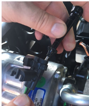
FIGURE 2: PED CONNECTOR EXTRACTING TOOL
