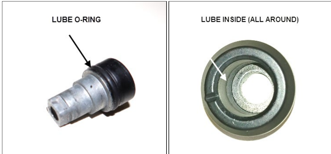
FIG.7 CYLINDER LOCK LUBRICATION POINTS
