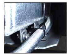
9. Insert the "GROMMET" into the existing hole of the frame as shown.
