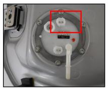
4. Measure the resistance of the sending unit's with the float in the low position.
