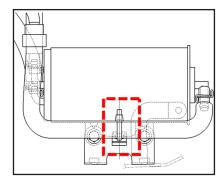
8. Install the "CANISTER" on the "BRACKET, CANISTER."
