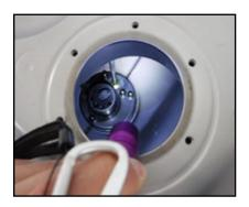
If there is rust in the fuel tank, replace it with a new one. Be sure to install new graphics, warning label, and dampers.
