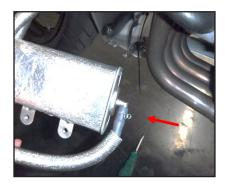
7. Put the "CLAMP" (zip tie) through the "BRACKET, CANISTER" as shown.
