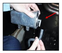
3. Assemble the parts from the kit as shown below by sliding the "PROTECTOR, PIPE" over "PIPE, 4" and connecting "PIPE, 5" using the "JOINT."
