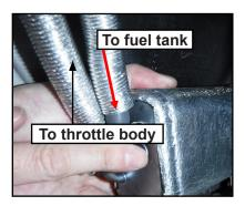
6. Attach the newly assembled "PIPE, 4" from step 3 to the opposite side of the canister as shown.
