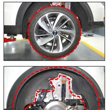
2. Remove the left rear fender liner.
