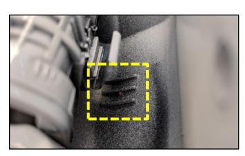
Slide the PC pad (Side B) faced down over the fuel door marking. Press down firmly (Side A) to ensure pad is flat against the fuel door surface.
