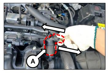
Release the fuel pressure by referring to the "Engine Control / Fuel System → Fuel Delivery System → Repair procedures (Release Residual Pressure in Fuel Line)" chapter in the applicable Shop Manual on KGIS.
