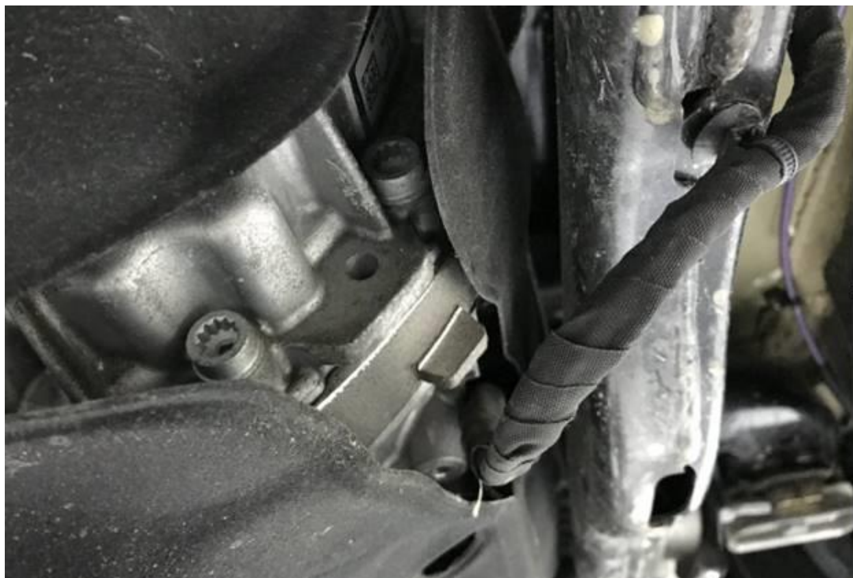
Figure 7. Final harness routing.
