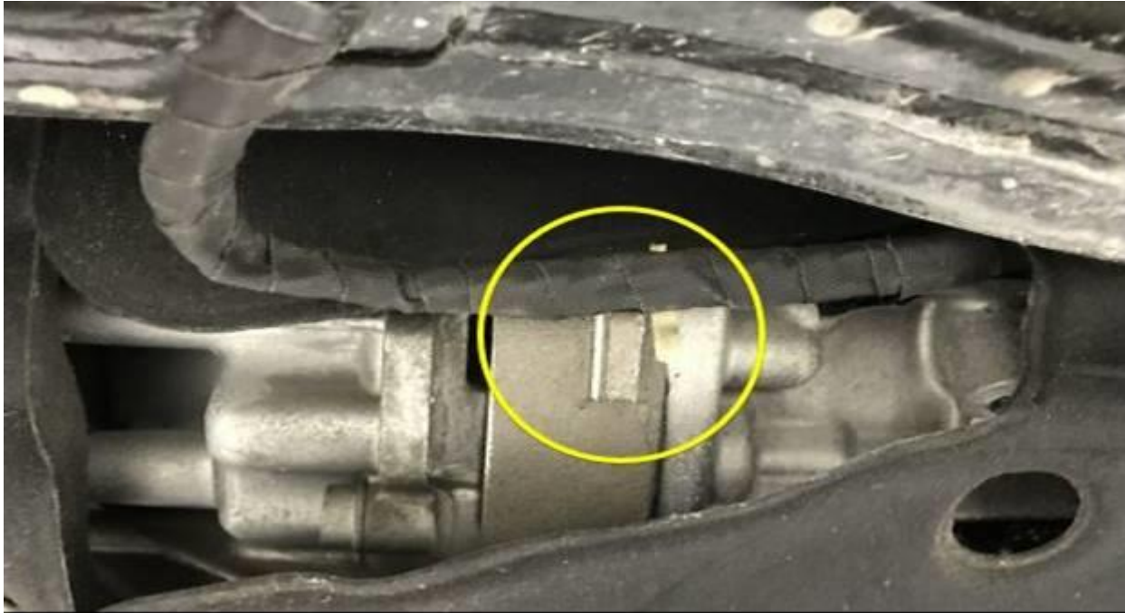
Figure 4. Harness may be routed under the lugs (Figure 3) or over the lug.
