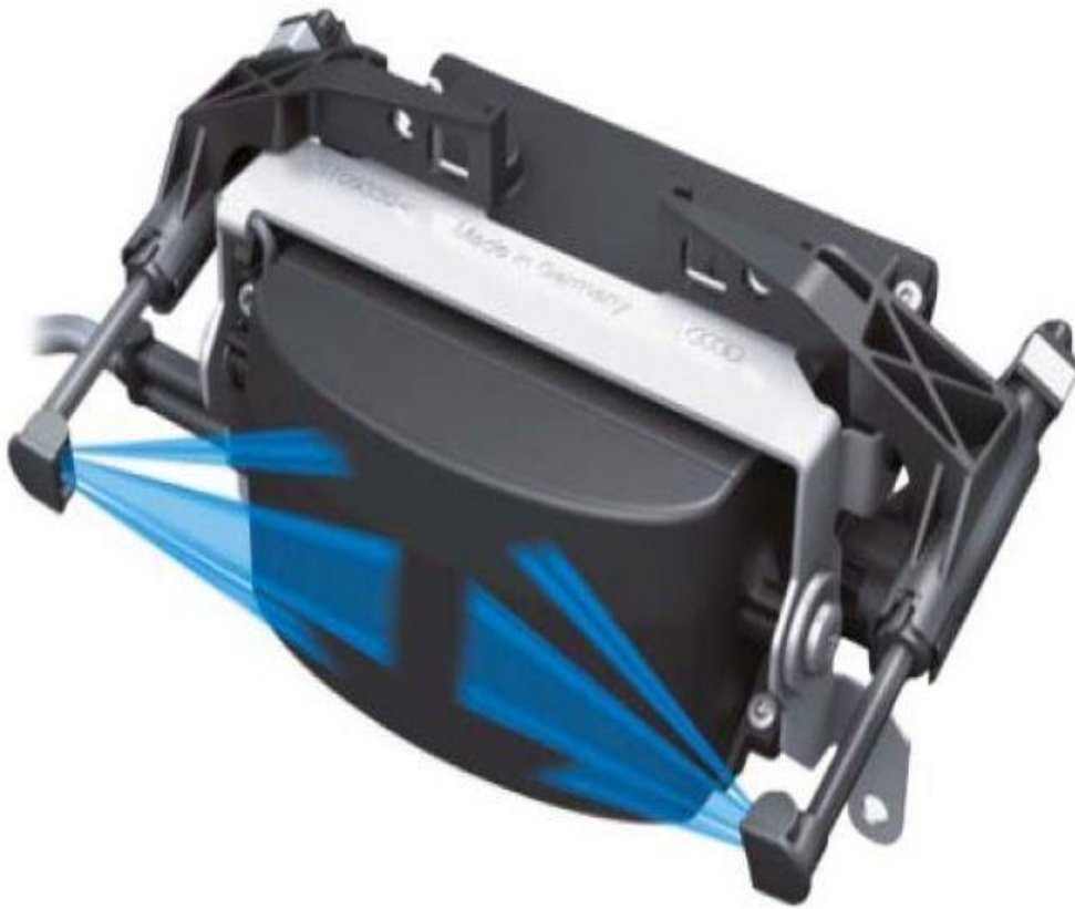
Figure 1. Laserscanner cleaning system.
