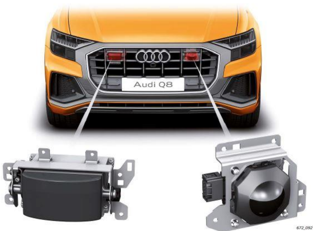
Figure 2. Laserscanner locations (A6, A7, and Q8).
