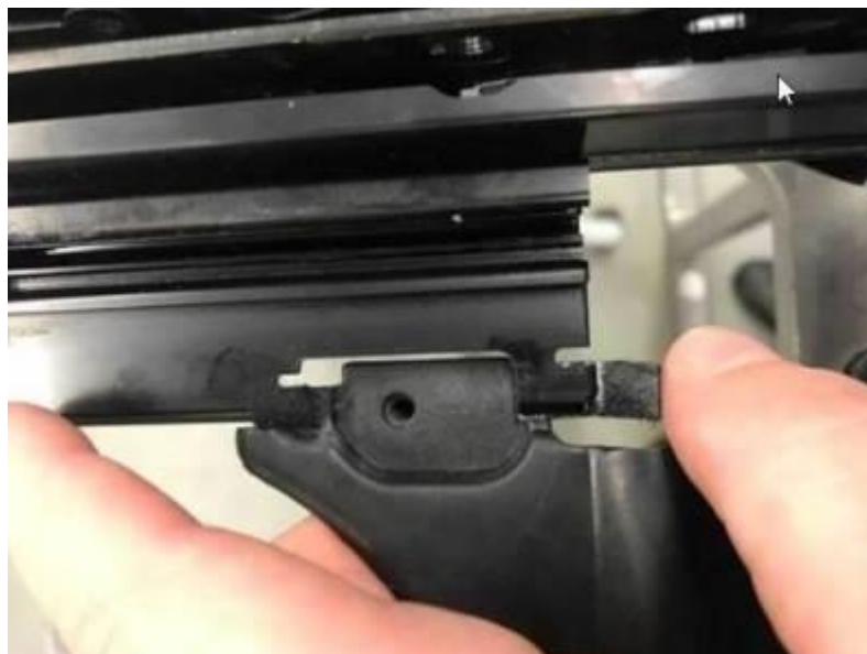
Figure 7. Areas to clean using cleaning solution D 009 401 04.
