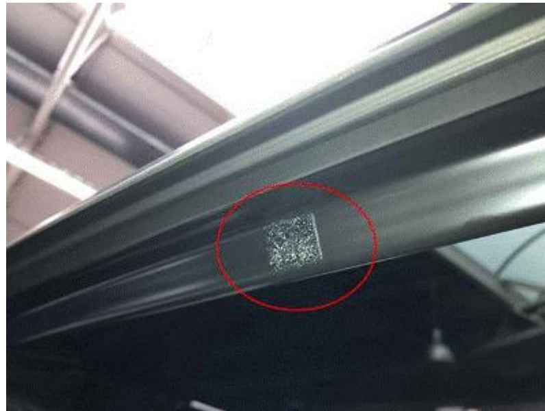
Figure 17. Adhesive felt strip material affixed to the center area of sunroof glass panel structure.
