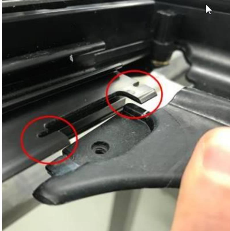
Figure 7. Areas to clean using cleaning solution D 009 401 04.
