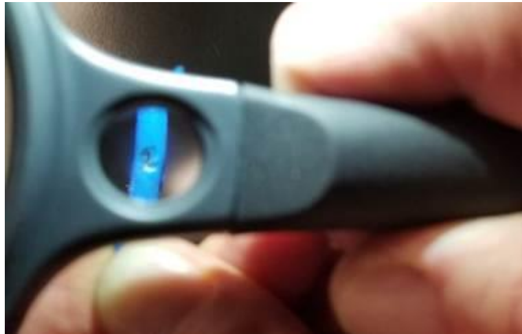
Figure 4. The cause of the DTC may be as small as a pinhole.
