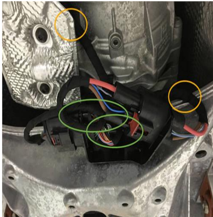
Figure 1. Common areas for harness damage.
