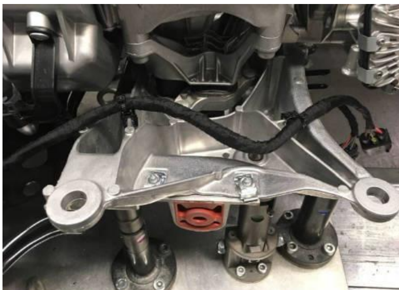
Figure 6. Routing and mounting of the transmission harness behind the crossmember.
