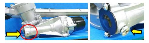
**Step 3-** Remove the tension spring and replace with the new part. Make sure the new spring is fully seated in the hole.
