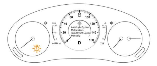
If the rain sensor detects temperature higher than the operation range, the auto light system temporarily stops and the exterior light warning indicator light turns ON.
