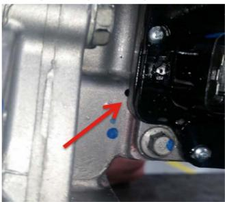
When fluid is found to be leaking out of or near the right side weep hole on the PTU, validate if the leak is from the weep hole or the actuator sealing surface.
