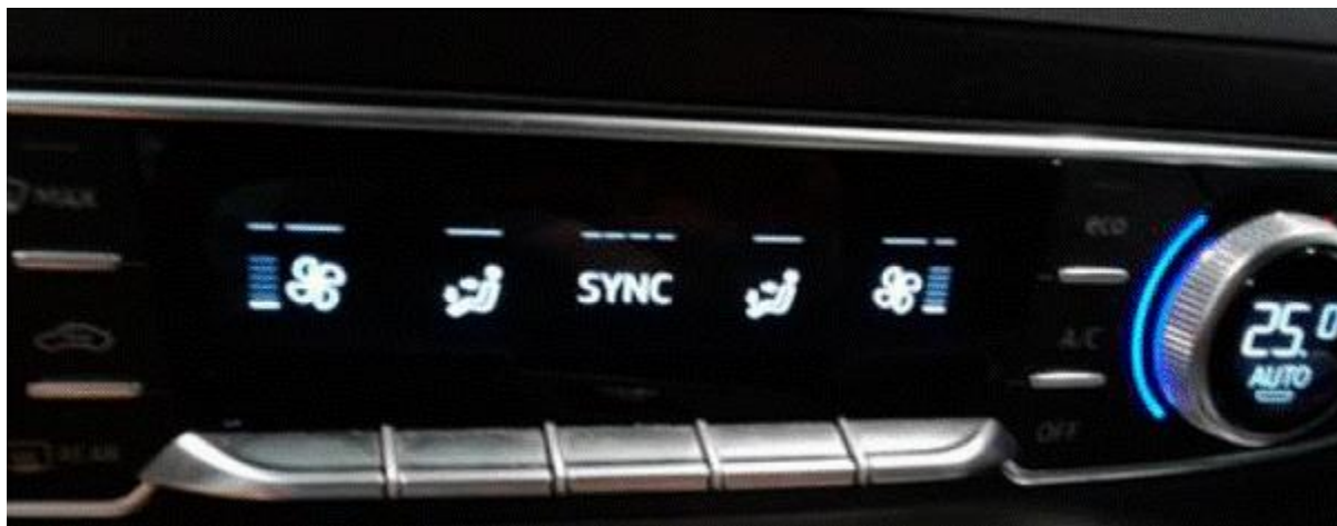
Figure 1. Display clarity is not sharp or may be missing segments.
