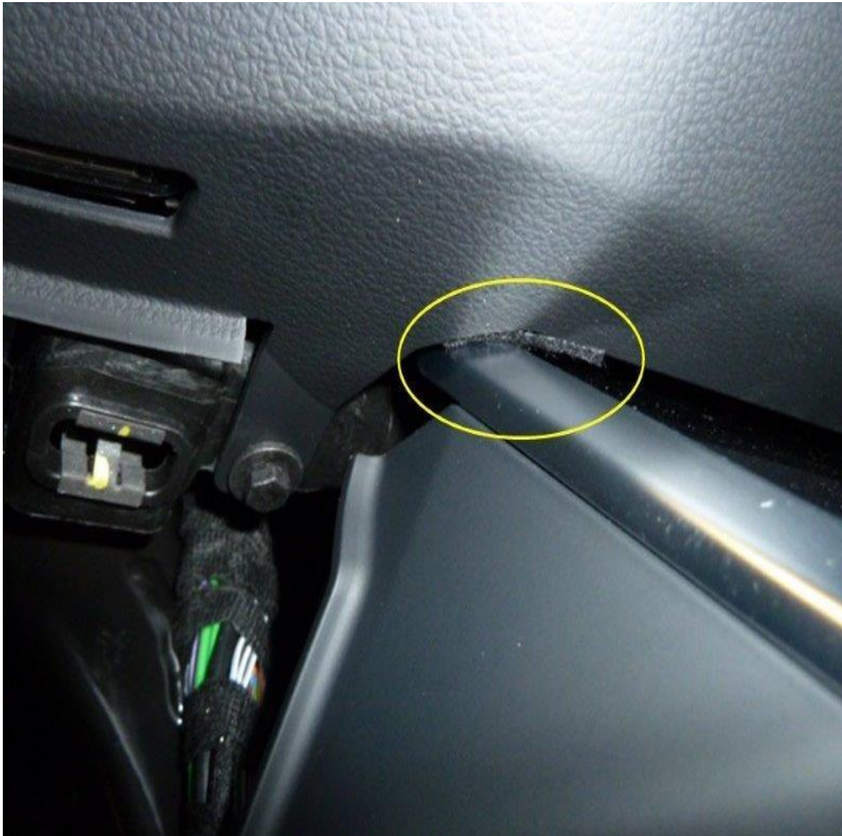
Figure 1. Installation of the felt strip shown (yellow circle).
