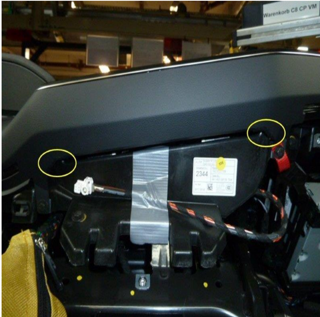
Figure 2. Positions of the felt strips (yellow circles).
