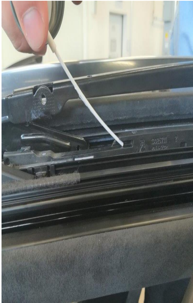
Figure 6. Lubricating the groove in the slide and tilt mechanism.
