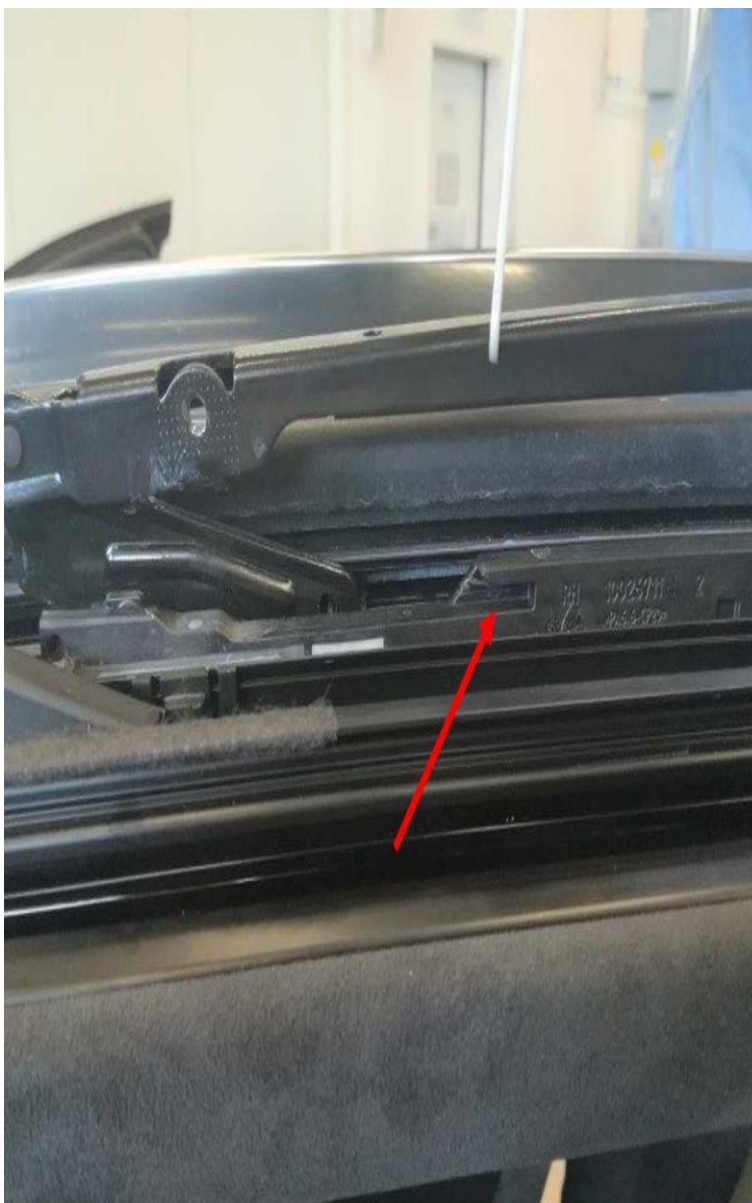
Figure 5. Groove in the slide and tilt mechanism.
