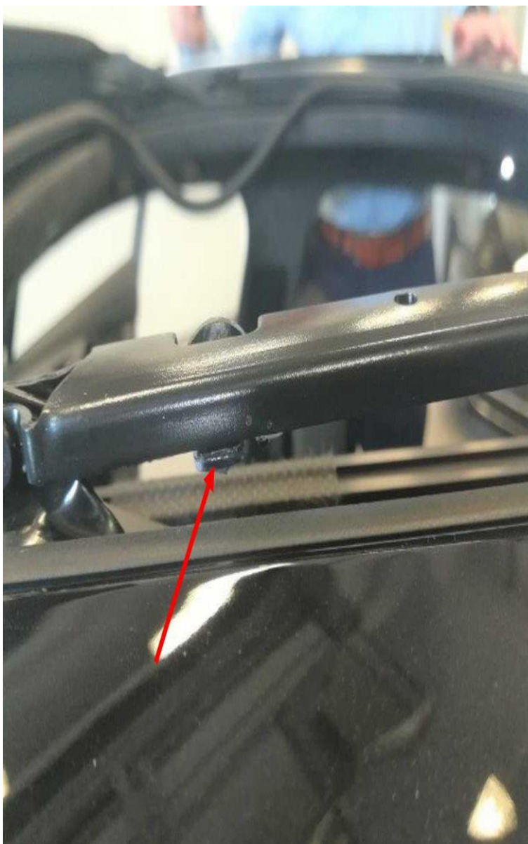
Figure 4. Lug to be lubricated on slide and tilt mechanism.
