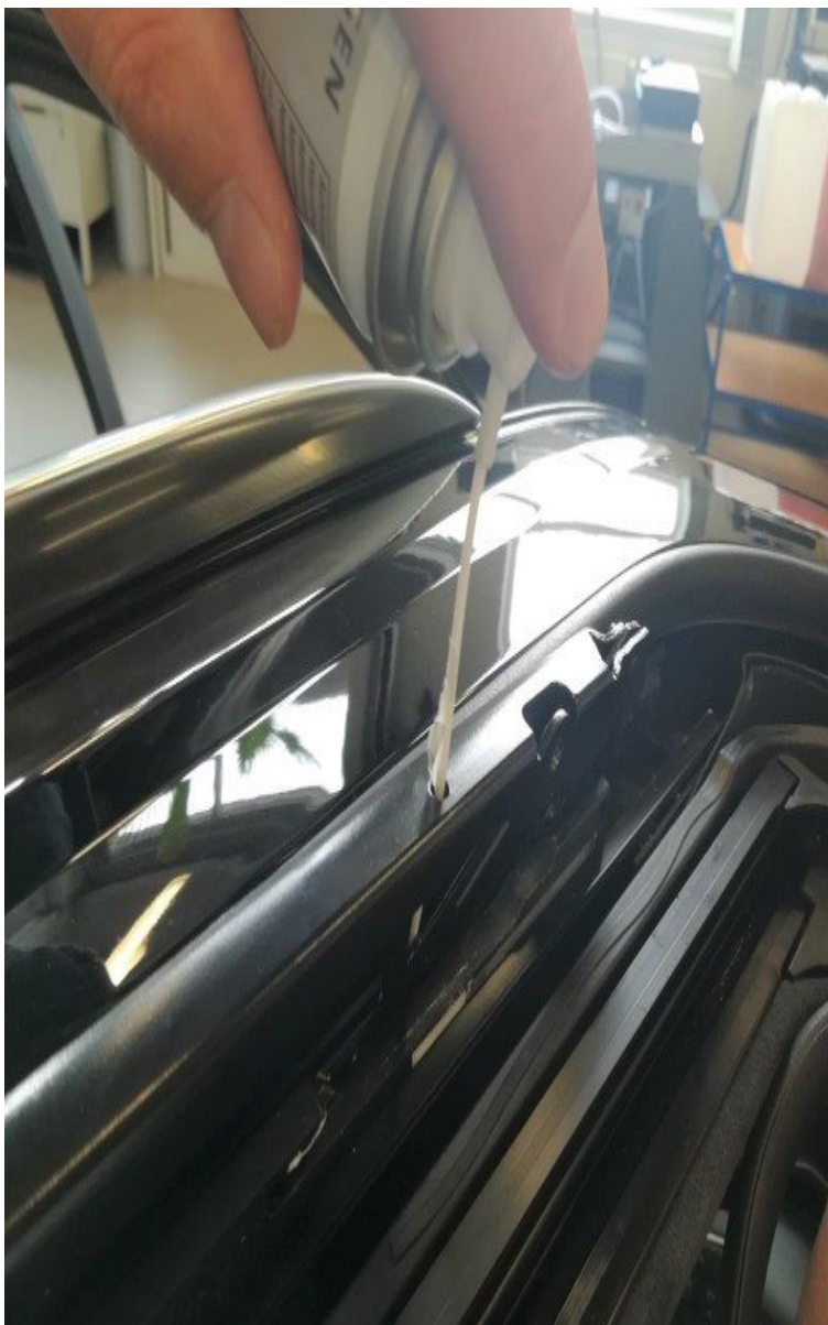
Figure 9. Accessing the channel through the arm of the slide and tilt mechanism.
