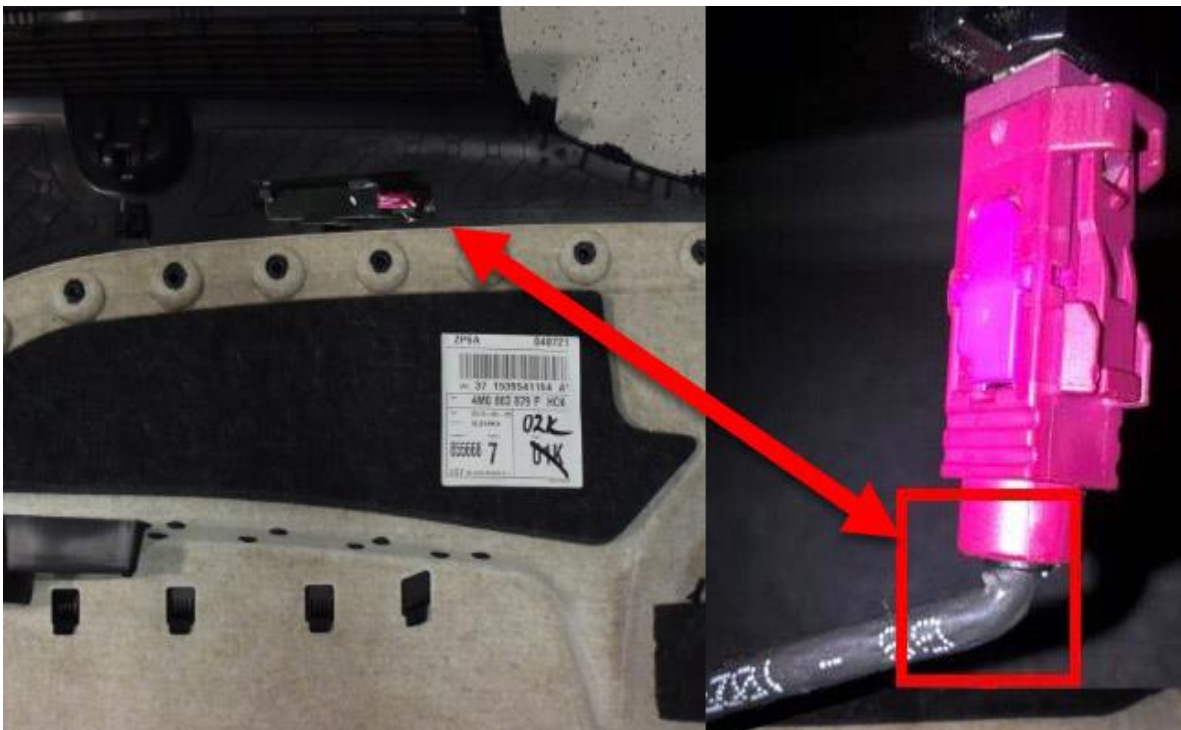
Figure 2. Coaxial wire kinked at R263 SOS Antenna.
